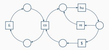
(P,T,F,l) P,T disjoint and finite sets  $F\subseteq (P\times T)\cup (T\times P)$   $l:T\to \Sigma \text{ ($\Sigma$ is an alphabet)}$
