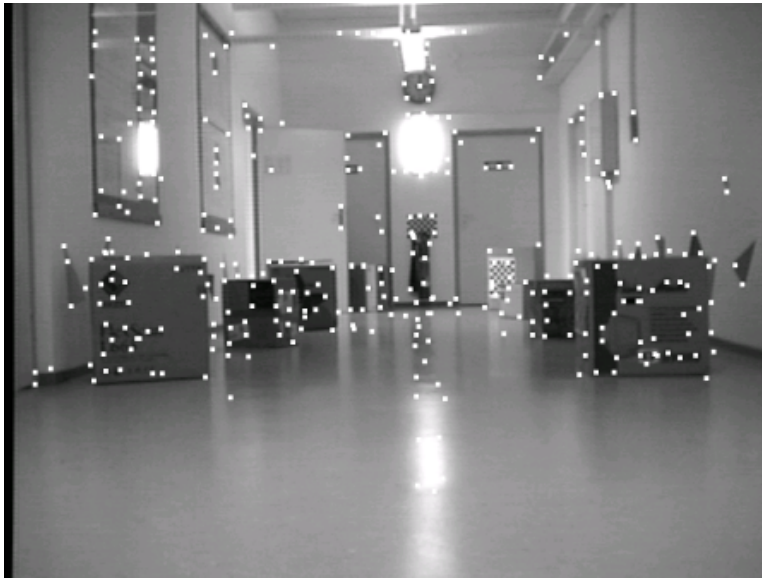
Figure 3.4: A 640 \times 480 image acquired by the robot's CCD camera. The locations of the features that were found are indicated by filled white rectangles.
