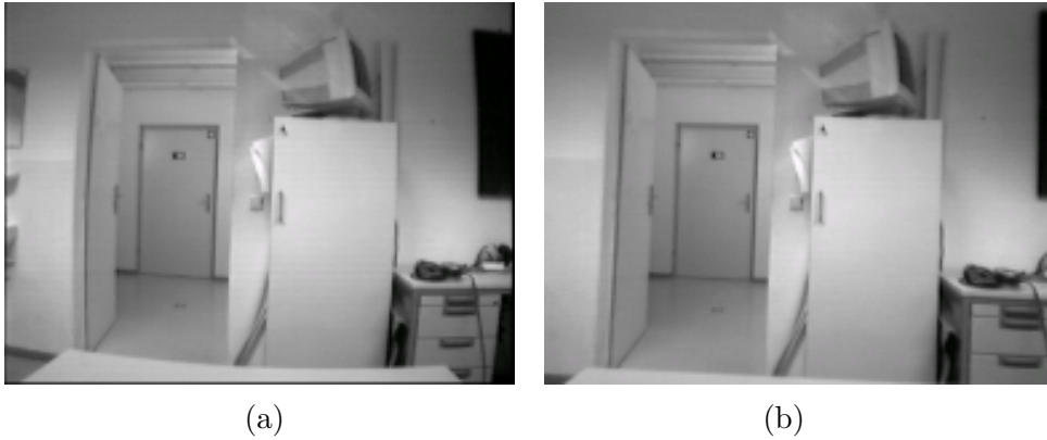
Figure 2.2: (a) An image from a simple CCD camera. Radial “barrel” distortion is clearly visible. (b) The same image with radial distortion removed. Now straight lines in the world appear as straight lines in the image, e.g., the door frame on the left or the edge of the blackboard on the right.
