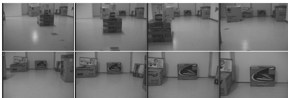
Figure 6.9: Some images acquired by the robot camera during the “navigation” experiment. Since natural visual features in the scene are sparse, several cardboard boxes have been placed on the floor.
