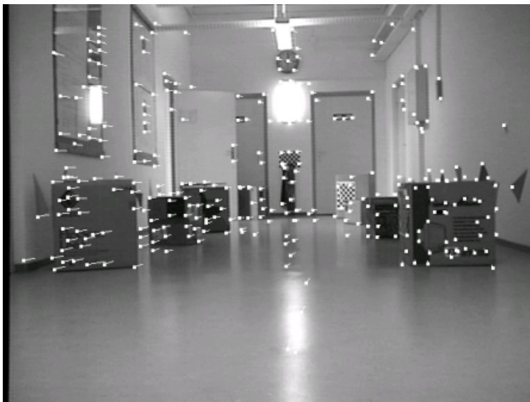
Figure 3.5: The features that were selected in Figure 3.4 were tracked in the next image of the sequence. Filled white rectangles are placed at the current feature positions. The white lines indicate from which locations in the previous image the features were tracked.
