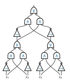
Parity function with four inputs: (true for odd number of 1s)
