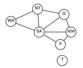
General-purpose CSP algorithms use the graph structure to speed up search. E.g., Tasmania is an independent sub-problem!
