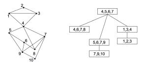
Width: max(vertices in tree node)-1 = 3. Treewidth: minimal width over all possible tree decomposition.
