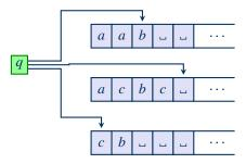
**Definition 2.9:** Let  $k \in \mathbb{N} \setminus \{0\}$ . Then a (deterministic) k-tape Turing machine is a tuple  $\mathcal{M} = (Q, \Sigma, \Gamma, \delta, q_0, q_{\text{accept}}, q_{\text{reject}})$ , where
