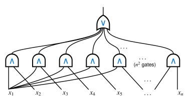
Corresponds to formula  $(x_1 \wedge x_2) \vee (x_1 \wedge x_3) \vee ... \vee (x_{n-1} \wedge x_n)$   $\sim$  accepts all strings with at least two 1s
